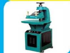
Non-Woven Fabric Grinding Machine
